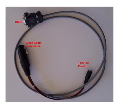
This cable can be used to connect to the SCC Sensor to Power and a PC directly without the need for the Display / Interface.
