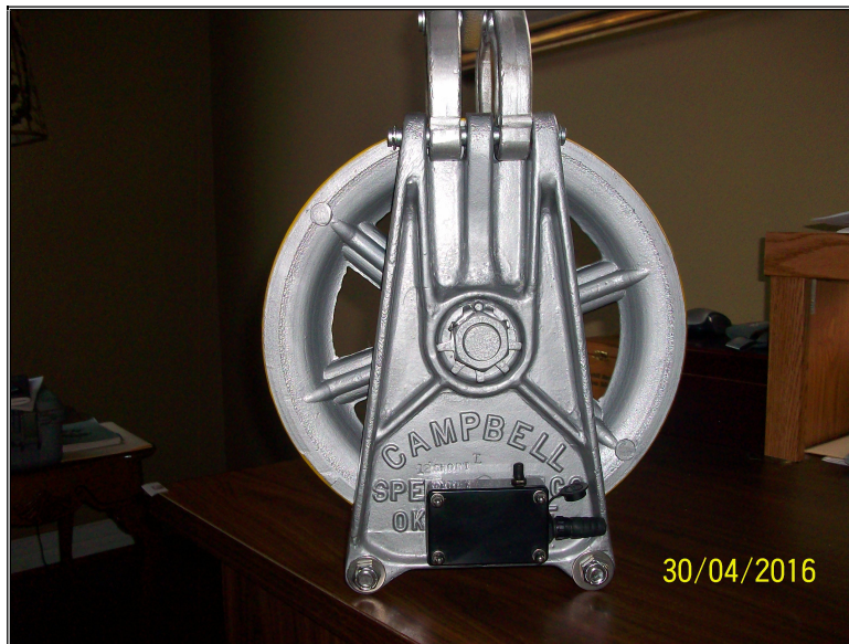
The SCC BT Sensor mounted to Campbell 12" Sheave Block
